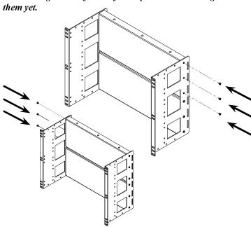
Step 4 nstall Bottom Cover Panel. Place cover panel with flange facing up and short depth side cut facing forward as in illustration. Secure side brackets with (3) M4 screws to right and left side of cover panel but do not tighten them yet.
