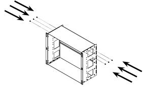
Step 6 Tighten all M4 screws on both right and left hand side. Makes sure all panels and brackets are secured and not moving. Assembly complete.
