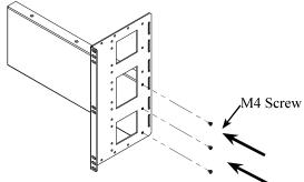
Step 2 Install Left Side Bracket. Secure side bracket with (3) M4 screws to bottom panel but do not tighten them yet.
