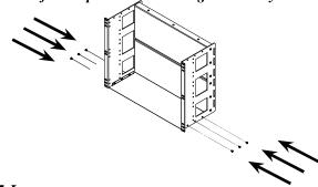
Step 5 Install Bottom Cover Panel. Place cover panel with flange facing down and short depth side cut facing forward as in illustration. Secure side brackets with (3) M4 screws to right and left side of cover panel but do not tighten them yet.
