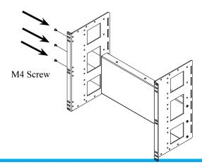
Step 3 Install Top Panel. Secure side brackets with (3) M4 screws to right and left side of solid panel but do not tighten than yet
